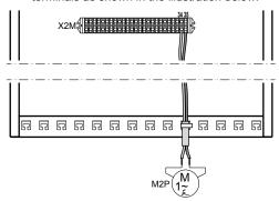
2 Fix the cable with cable ties to the cable tie mountings.
