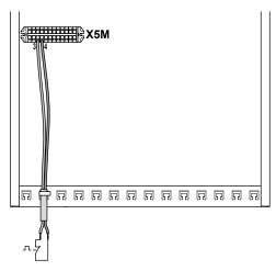
2 Fix the cable with cable ties to the cable tie mountings.
